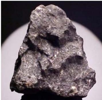
Cerussite, galena, and native silver were the principal ore minerals in the upper portion of the mine (and mined for silver and lead), while zinc-bearing sphalerite was more prevalent deeper in the mine.
